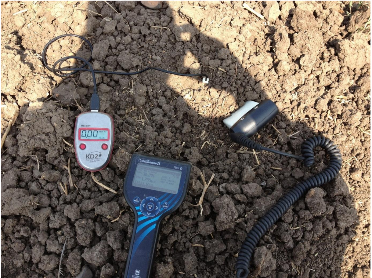
Figure 30 Measurement of soil moisture and soil thermal conductivity by HydroSense II and KD2 (Sakha, September 2012)
