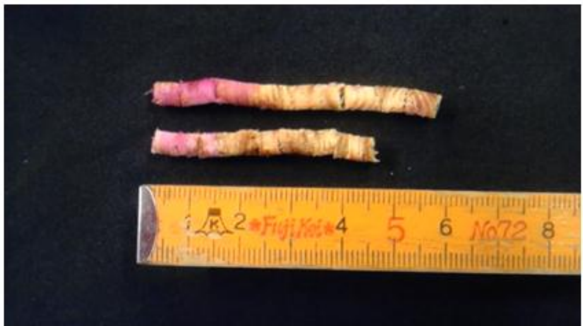
Figure 15 The photograph of core samples of trees taken by an increment borer in August 2010. Left sides of core samples are bark and the red parts were dyed with stains. (Shimizu, 2011)
