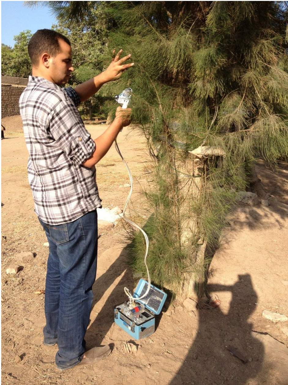
Figure 29 Measurement of tree's stomatal resistance by LI-1600 (Tomida farm, August 2012)
