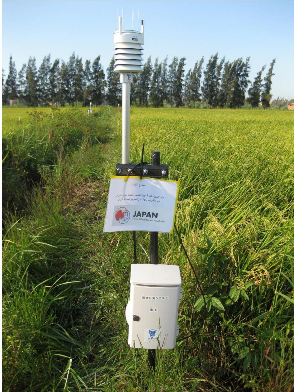
Figure 23 A set of Vaisala sensor for meteorological measurements (Al Krakat, August 2012)
